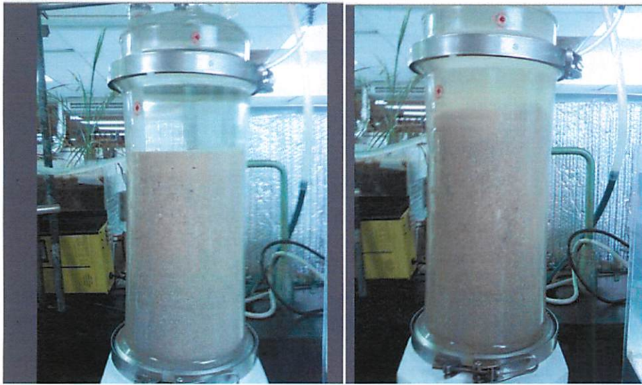
Photo 2. Sand bed expansion during the backwash (left: before the backwash; right: after the backwash).
