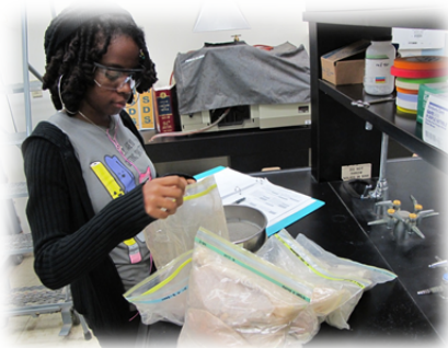
Figure 5. LEFT: Sediment samples being separated into a fine and coarse fraction. RIGHT: Furnace and crucibles used in LOI_{550} analysis.
