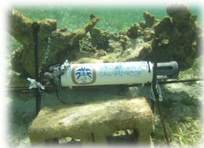
Figure 6. Sonde used to collect water quality parameters.
