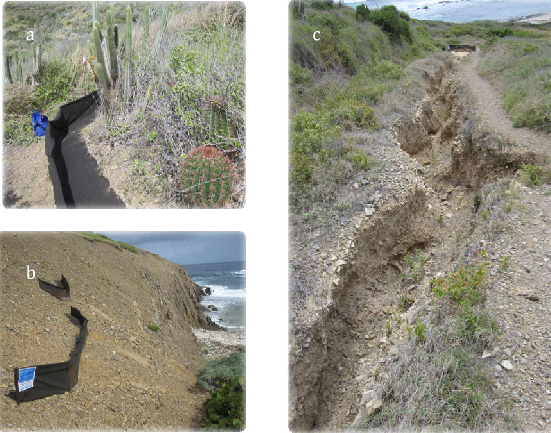
Figure 2. Representative sediment traps by surface type: a. vegetated hillslopes, b. cliffs and c. trail surfaces
