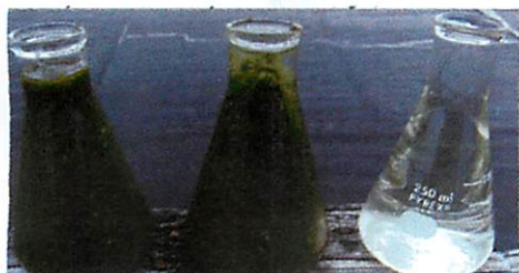
Figure 7. Comparison of untreated effluent (left), effluent treated with the polymer prior to entering the geotextile bag (middle), and filtrate exiting the bag virtually free of total suspended solids (right).
