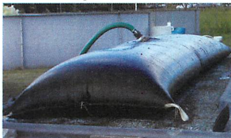
Figure 5. Filling the geotextile bag with aquaculture effluent injected with polymer. The slurry entering the bag will dewater as filtrate escapes and evaporation takes place. The bag can be filled multiple times.
